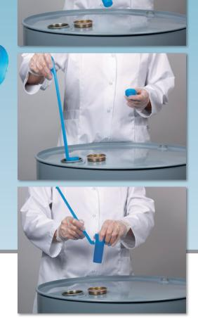
DispoDipper is completely manufactured in one piece and can be used for sampling and subsequent transport of the sample in one device. In this way, cross-contamination or sample impurities are almost impossible. After sampling, the handle at the predetermined breaking point can be detached from the sample container.
